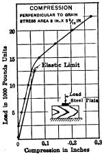
Fig. 6a.—Stress strain diagram for compression test.
